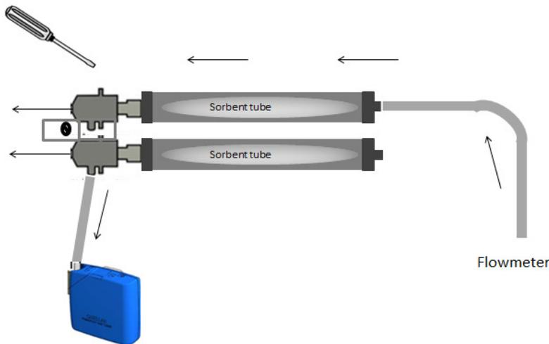
Break off both ends of the sorbent tubes and fit into the holder with the arrow pointing towards the pump. Connect the other to the flowmeter.
