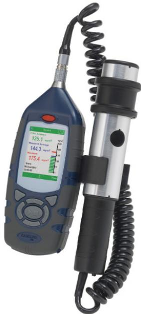
It has a simple calibration filter that can be used to provide a check of the instrument's linearity and has a large measuring range between  $0.001\text{mg}/\text{m}^3$  to  $250\text{g}/\text{m}^3$ . The instrument itself automatically ranges. The Microdust Pro logs the real time data which can be downloaded later for report writing.
