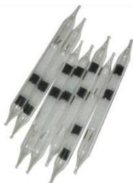
It is important to mount the tube so that the air flow through the tube is correct. Generally the smaller sorbent layer should be nearest the pump. Always ensure that the tube is near vertical during sampling and that there is a clear break at the end of the tube of at least 2mm in diameter to allow the drawing through of air.
