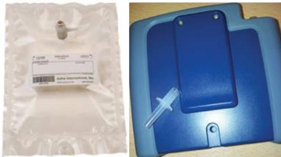
Attach the Tedlar bag to the outlet of the pump using a suitable length of tubing and a luer fitting e.g. Casella TUC12. In some pumps, the bag fill mode is automatic. Once the pump is set running, the pump will stop automatically when it senses the bag is full. If your pump does not have this feature, work out the time you need to fill the bag. Take care not to overfill the bag.
