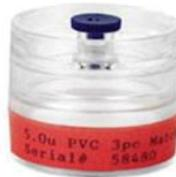
Each cassette contains two filters which are matched in weight within a tolerance ( $50\mu\text{g}$  for the MCE filters and  $20\mu\text{g}$  for the PVC filters). From the below diagram you can see that air is drawn in through the inlet and deposited on the test filter. There is a second filter underneath which acts as a blank. After sampling, both filters are equilibrated and re-weighed and the difference in weight is the amount of contaminant.
