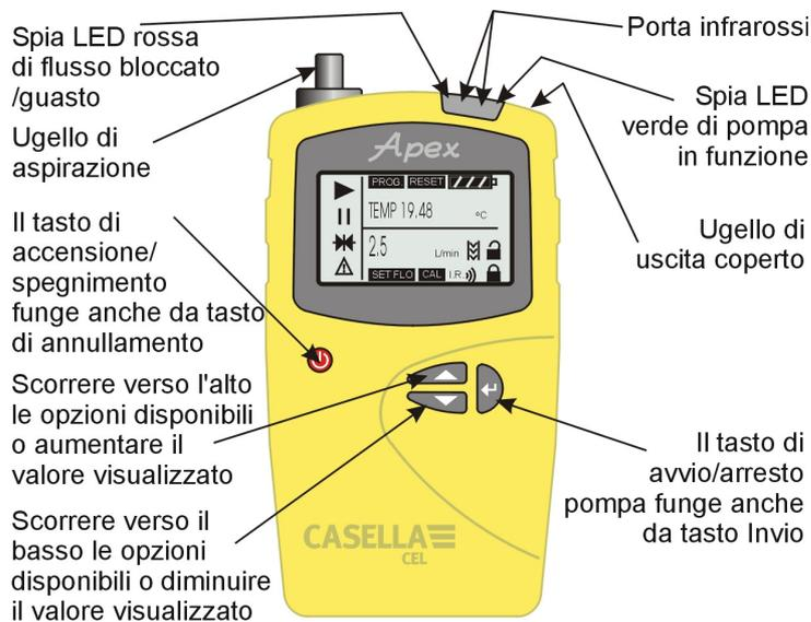
Figura 1: Pompa Apex
