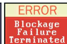
After one minute the pump will attempt to re-start. If the pump has not been able to re-start after the specified number of retry attempts, the pump will terminate the current sampling run and display an error message.
