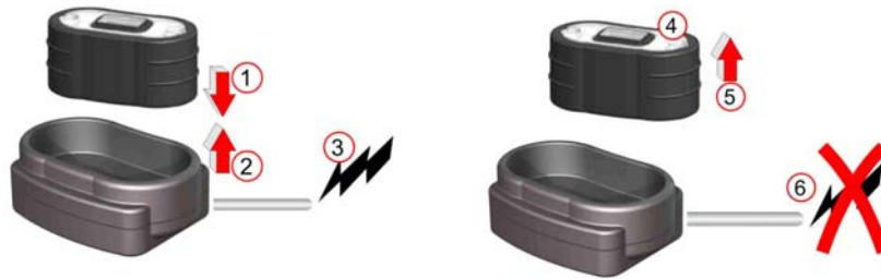
Figure 3 Insert Battery in Charger
