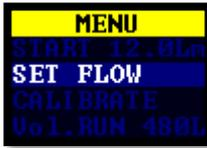
This is the menu that you use on a regular basis to set the flow and calibrate the pump between sample runs. It also gives you the ability to pre-select a sample volume or perform a timed run (see *Setup before starting a run* on page 13).
