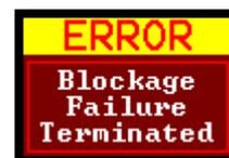
After one minute the pump will attempt to re-start. If the pump has not been able to re-start after the specified number of retry attempts (see Settings, page 19), the pump will terminate the current sampling run and display an error message.
