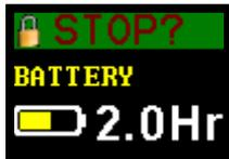
Full lock mode is denoted by a closed padlock icon and can only be set when the pump is running. While in full lock mode, the keypad is fully de-activated, and the user cannot stop or disturb the pump by any key presses.
