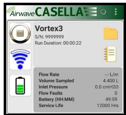
To save power, the Airwave Software stops scanning when all instruments within range have been detected.
