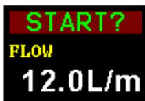
This is one of five dashboard screens that can cycle after you turn on the pump. The same information is also displayed when the pump is running (see *Operation* on page 12).
