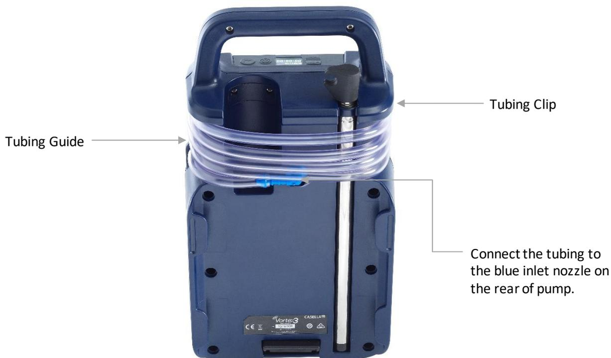
There is convenient stowage for a sampling head and tubing. Remove the sampling head (if already fitted) from its stowed position and unwind the tubing noting that there is a clip just below the handle and a guide to 'manage' the tube where it connects to the inlet nozzle.
