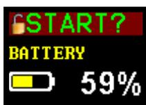
Partial Lock mode is denoted by a half open padlock icon and can be set in **Run** or **Stop** modes. While partially locked, the user may stop and start the sampling pump but has no access to the menu or other functions.
