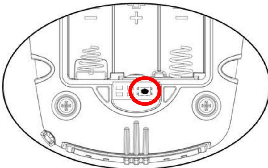
7. Press the Program Mode Switch using a non-conductive instrument and hold it down while simultaneously pressing and holding the instrument power button. Click 'Search For Devices' to locate the instrument to be upgraded.
