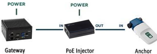
The POE Injector can be placed next to the Gateway it can also be affixed on the wall if required. Mains power is supplied to both the Gateway the POE Injector using the mains supplies provided.
