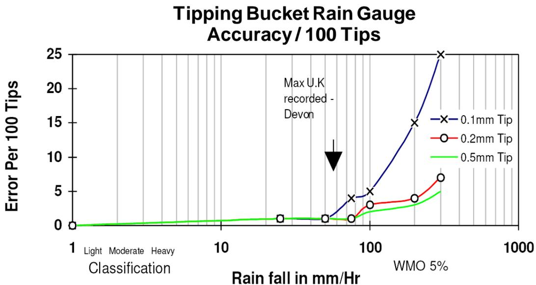
Figure 2: Accuracy of 0.1 mm, 0.2 mm and 0.5 mm tip versions
